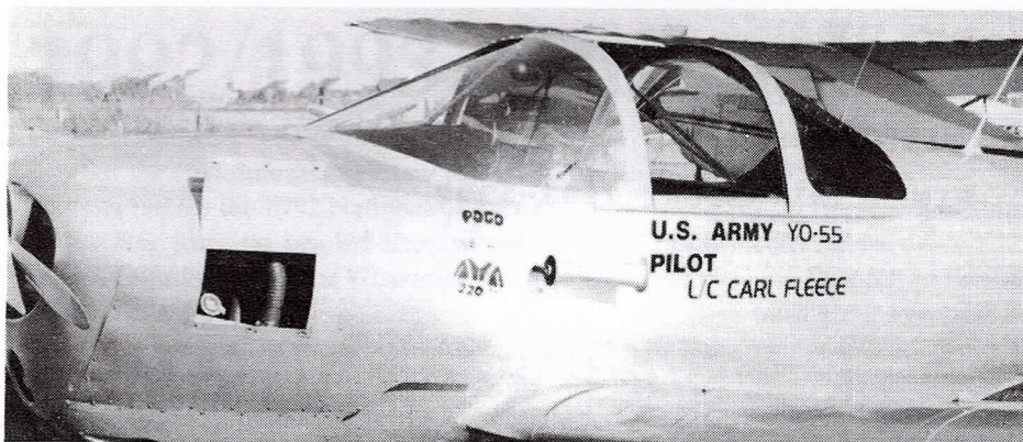
After removing the fuselage fuel tank, Carl Fleece installed two Forney fuel tanks in the wings, outboard of the regular wing tanks. Note the new gradually sloping "flat" windshield.
